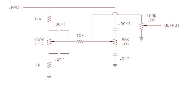
NOTE: SOURCE IMPEDANCE AT INPUT SHOULD BE LESS THAN OR EQUAL TO 1K.
